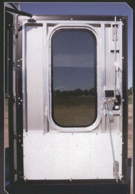
The lower inner door panel protects the outer door panel from damage caused by shifting cargo.
